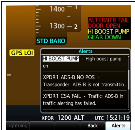
HIGH BOOST PUMP ALERT & ANNUNCIATION
