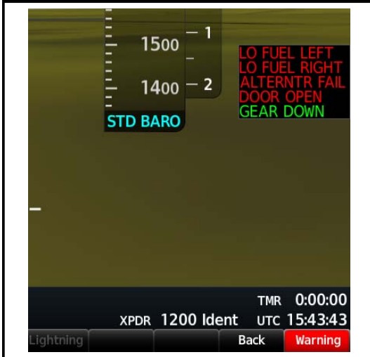
LOW FUEL WARNING - LEFT & RIGHT MASTER WARNING
