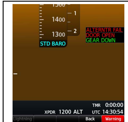
ALTERNATOR FAIL MASTER WARNING
