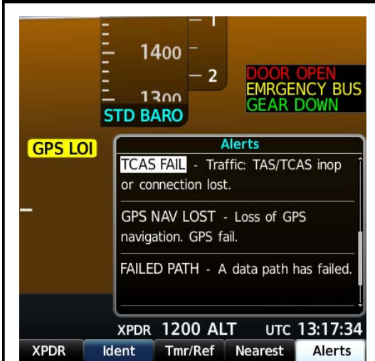
TCAS FAIL / DATA PATH FAIL
