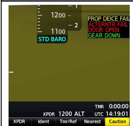
PROP DE-ICE FAIL MASTER CAUTION
